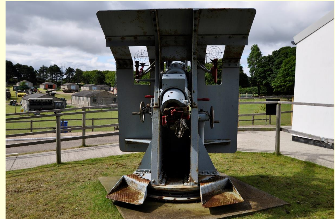
Fig. 14 Naval High-angle 12 pdr gun in the Muckleburgh Military Collection, Norfolk. HMT Chiltern had a single weapon of this type as her main armament. The gun was located forward of the main mast in the position of the two lifting 'A' frames (see Fig 13 left)
